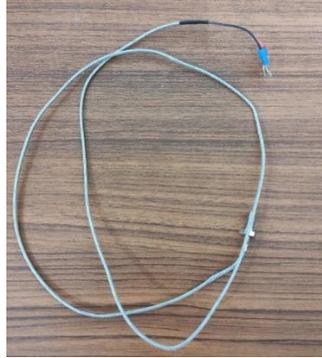
Gambar 3. 5 *Thermocouple*
