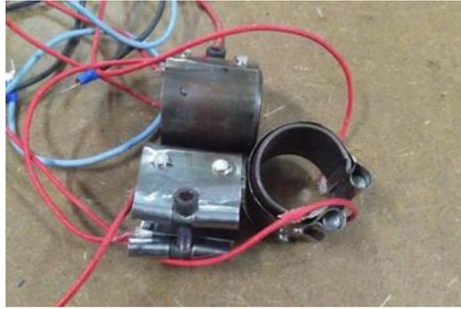
Gambar 3. 7 Heater Band 220V
