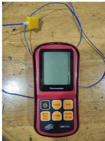
Gambar 3. 15 Thermometer Digital tipe K
