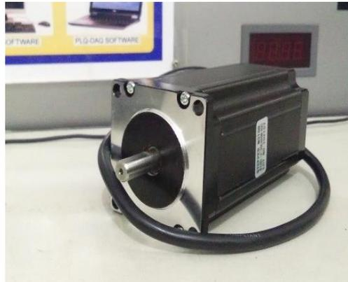
Gambar 3. 9 Motor Stepper Nema 23 Torsi 3 Nm
