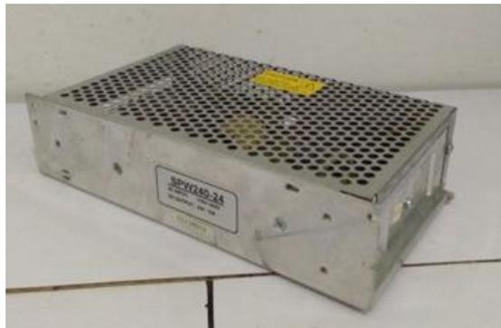
Gambar 3. 13 Power Supply 20V 10A
