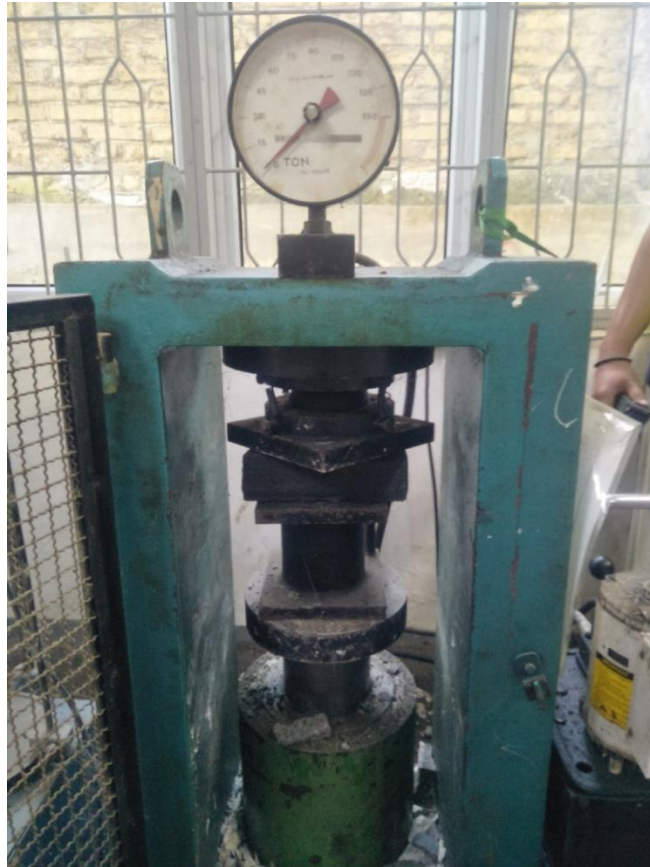
Gambar 4.9 Mesin Compression test
