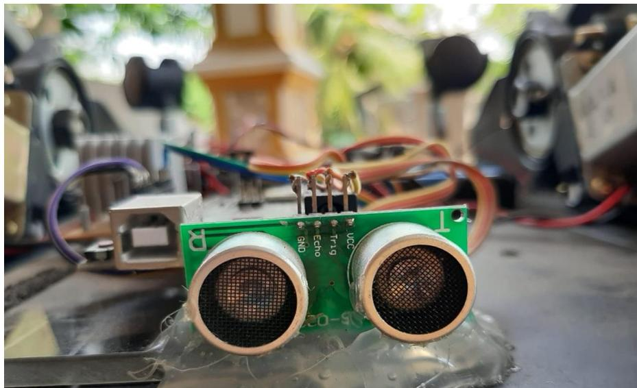
Gambar 2.9 Sensor Ultrasonic HC-SR04
