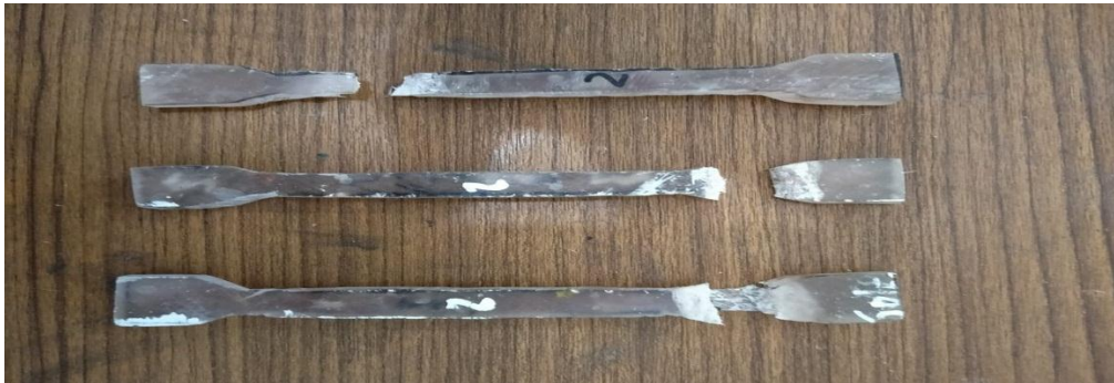
Gambar 4.2 Hasil Pengujian Tarik 50 % Resin : 50% Fiberglass
