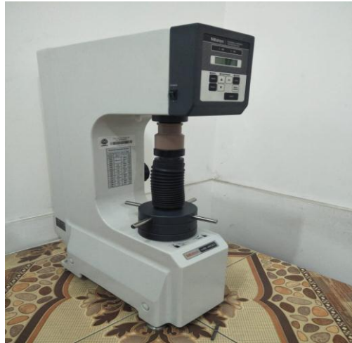
Gambar 4.21. Alat uji Rockwell (model mitutoyo HR-400)
