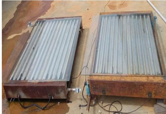
*Solar water heater double slope*
