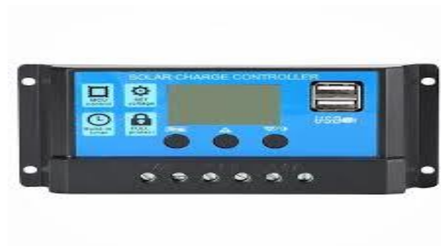
Gambar 2.11. Solar Charger Controller
