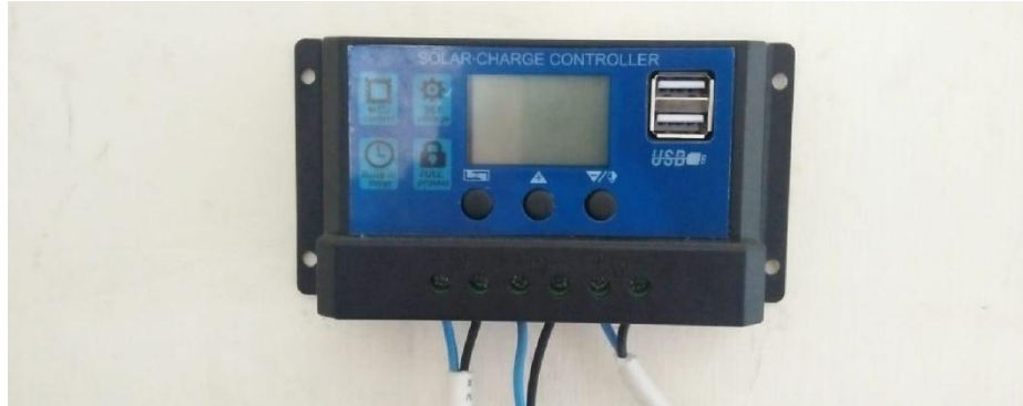
Gambar 3.2 Solar Charger Controller
