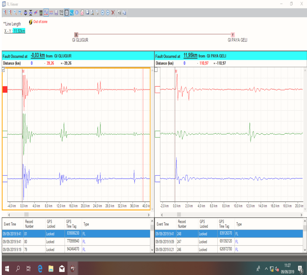
Gambar 2.9 Commissioning TWS FL 8 Glugur – Paya Geli 1
