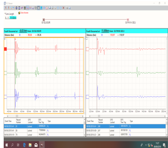
Gambar 5. Commisioning TWS FL8 Glugur- Paya Geli 1
