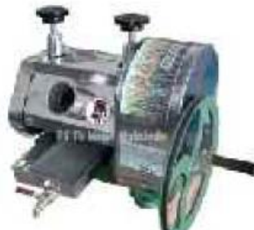
Gambar 2.1 Mesin peras tebu manual (Sumber;jurnal Harun Doe, Yunita Djamalu, Burhan Liputo,2016)
