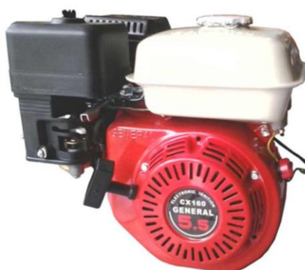
Gambar 2.4 Motor bensin 4 tak 5,5 hp (Sumber https://images.app.goo.gl/3knFLKmreeo1h5uq6 )
