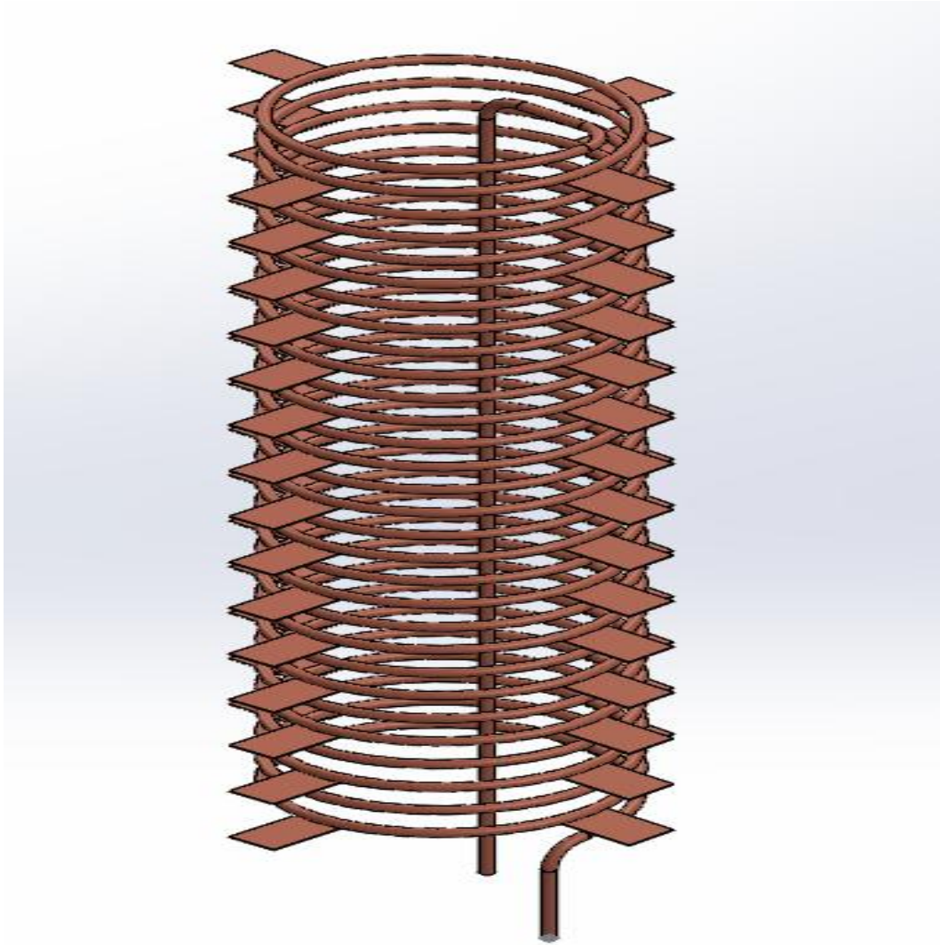
Gambar 3.29 Desain Sheel Helical Coil Bersirip 30 lilitan
