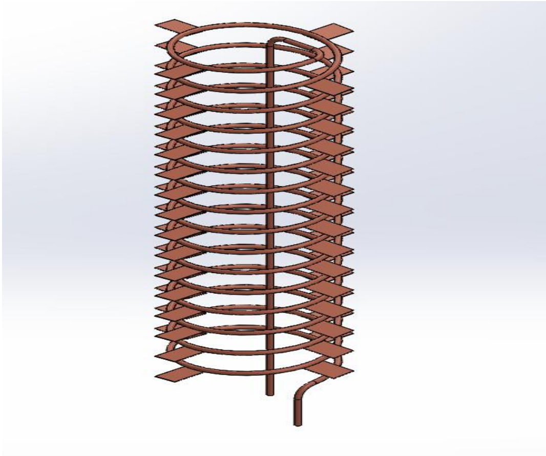
Gambar 3.15 Desain Sheel Helical Coil Bersirip 15 lilitan
