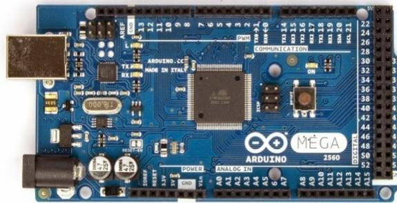
Gambar 2.4 Arduino Mega
