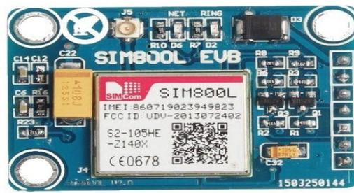
Gambar 2.15 Modul SMS Gateway
