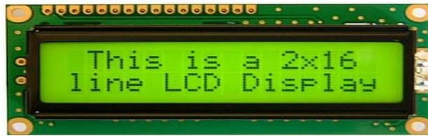
Gambar 2.13 LCD (Liquid Cristal Display)
