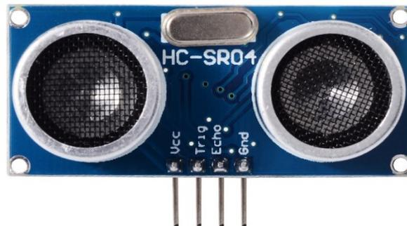
Gambar 2.12 Sensor Ultrasonik HC-SR04
