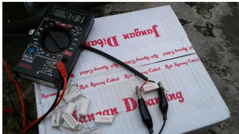
(a) Beban resistor 10 Ohms 5W
