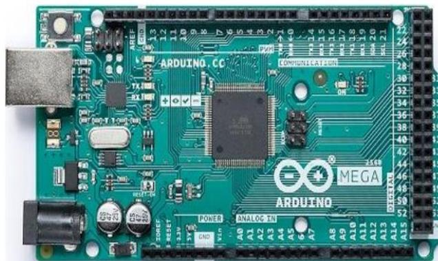
Gambar 2.11 Arduino Mega
