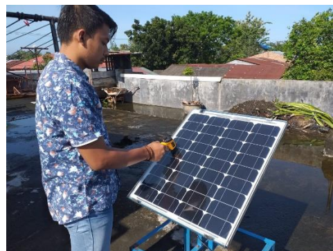
Gambar 3.28 Mengukur temperature panel
