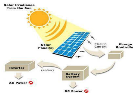
Gambar 2.8 Prinsip kerja Panel Surya (Yoga Pradona, 2019)
