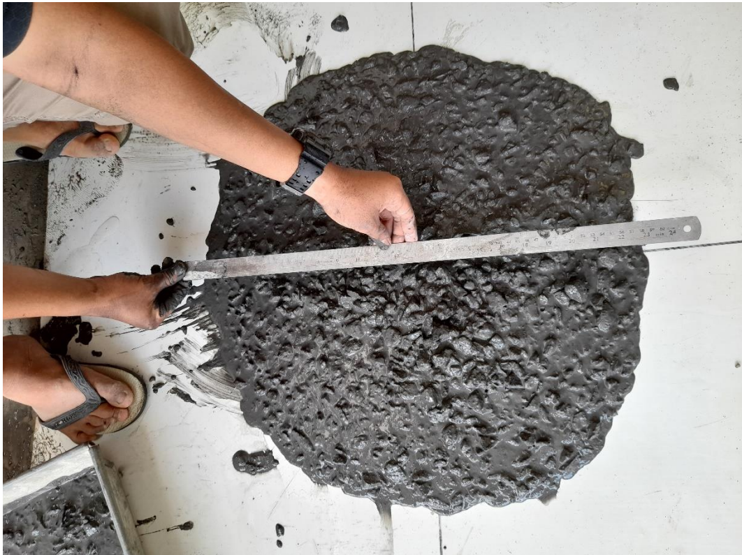
Gambar L-20: Pengukuran Diameter Slump Flow
