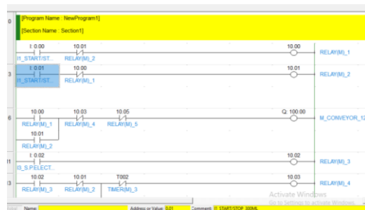
Gambar 3.21 Tampilan program input relay dan motor conveyor pengisian level 2
