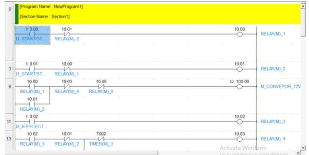
Gambar 3.21 Tampilan program input relay dan motor conveyor pengisian level 1
