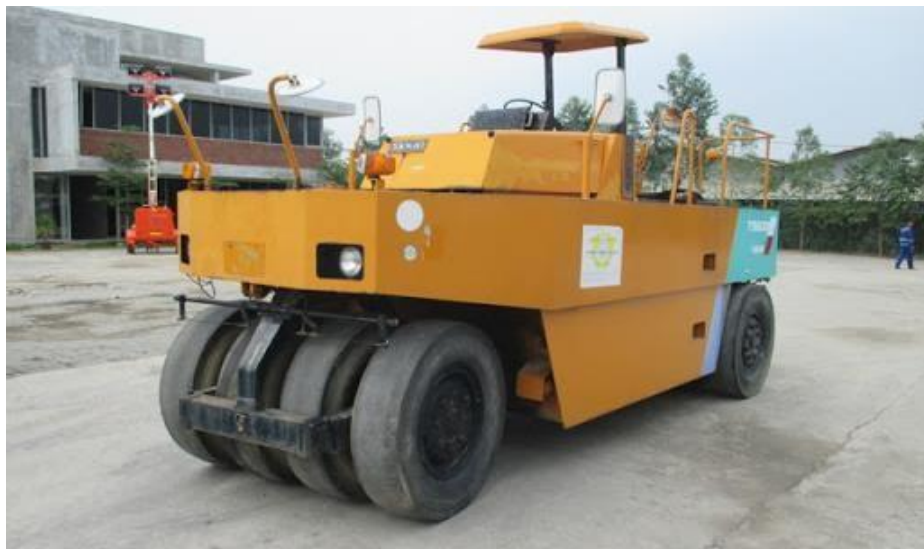
Gambar 2.8: Pneumatic Tyre Roller (Djoko Wilopo, 2009)
