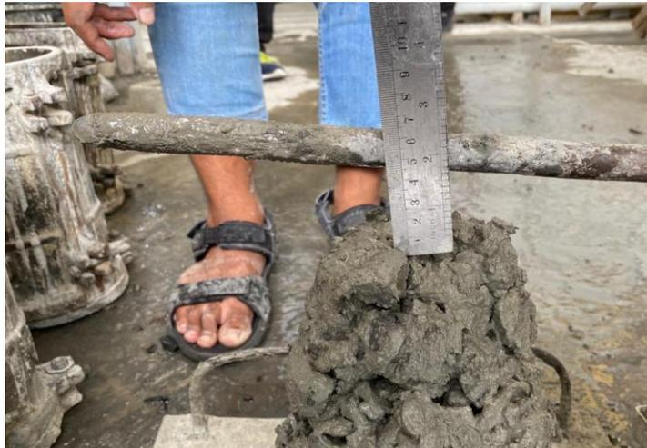
Gambar L-22: Pengujian Slump Test.
