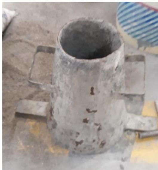
Gambar L-8: Kerucut Abrams.
