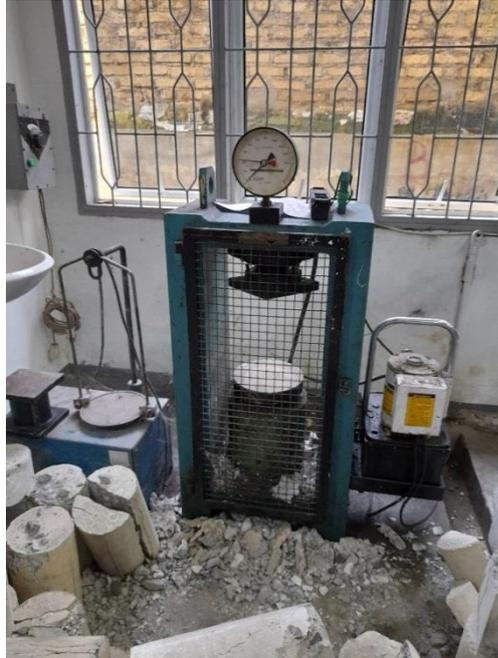
Gambar L-1: *Compressing Test Machine.*
