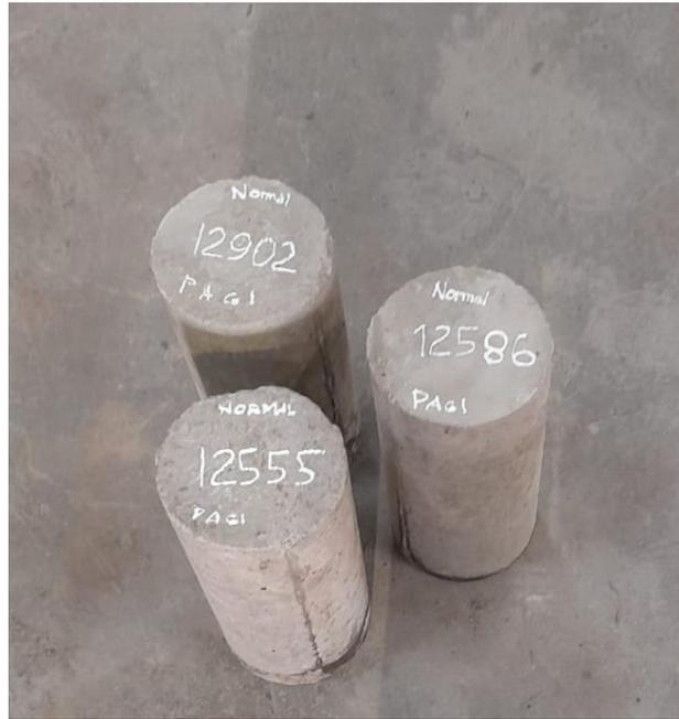
Gambar L-25: Beton Normal.
