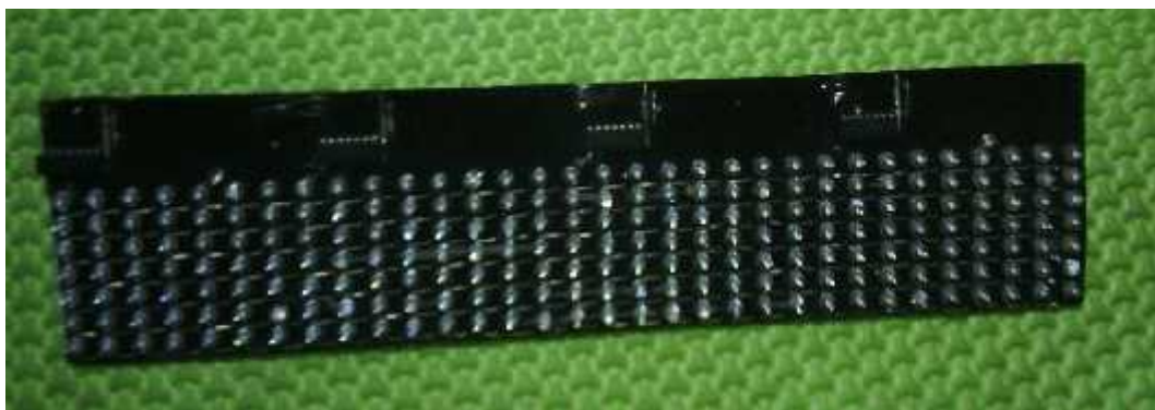
Gambar Hasil Pemasangan Rangkaian Driver LED Matrik
