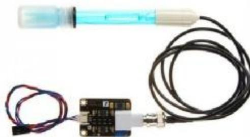
**Gambar 2.1** Sensor pH DZ-PHprobe
