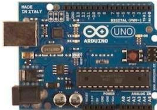
**Gambar 2.4 Board Arduino Uno**
