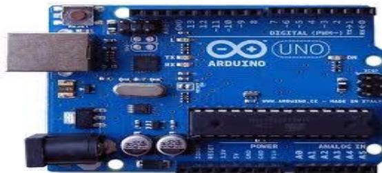
**Gambar 2.5. Board Arduino**
