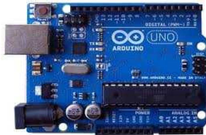
Gambar 2.3 Board Arduino
