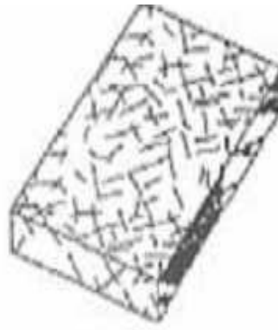
Gambar 2.6: Discontinuous Fibre Composite (chopped fiber composite)
