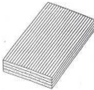
Gambar 2.4 Komposit serat kintiniu ( Continuous fiber composite ) (Gibson, 1995)
