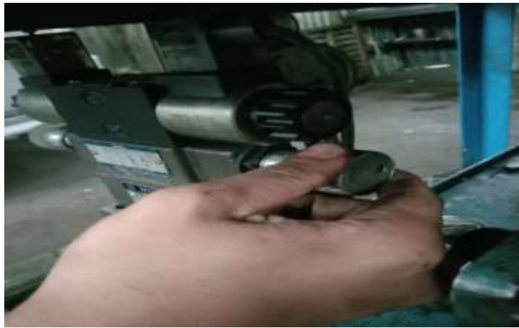
Gambar 4.7 Mengatur Throttle valve
