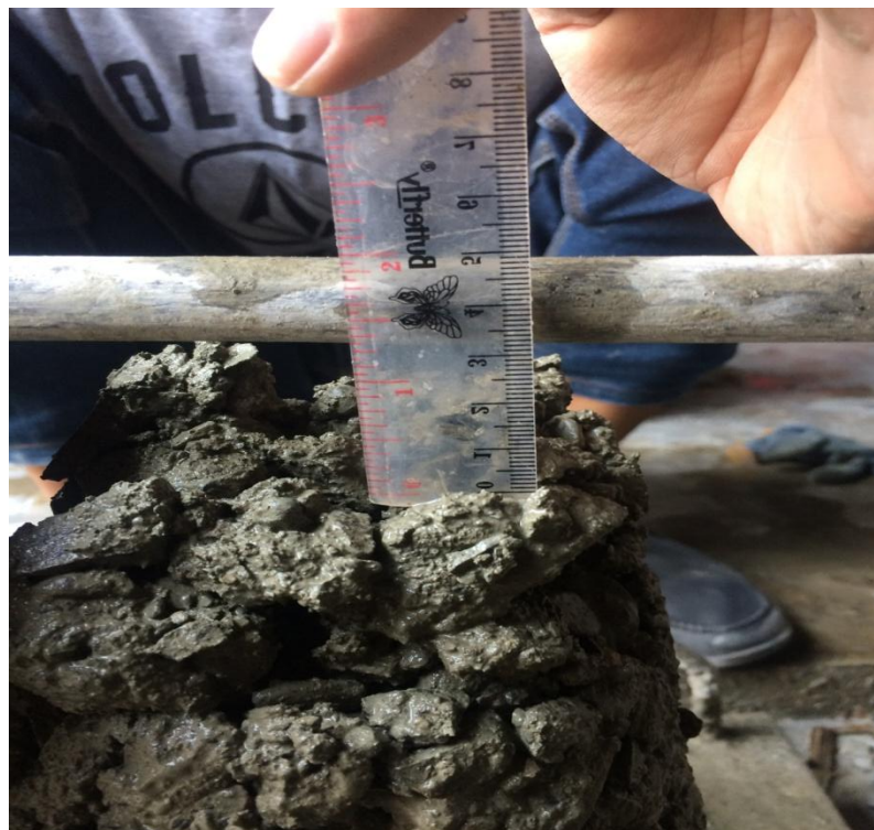
Gambar L6: Hasil pengujian slump test.
