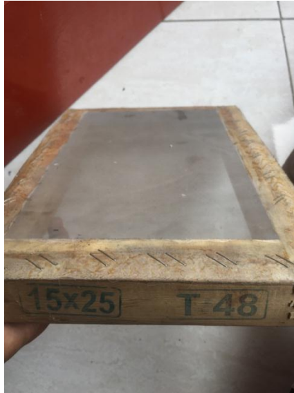
Gambar 3.7 Saringan T48 pengayak/filter.
