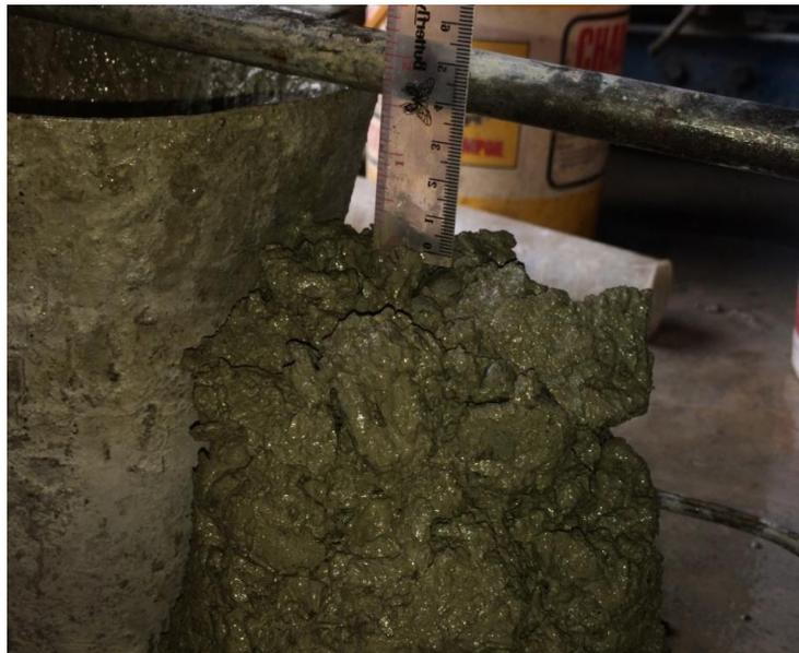
Gambar L8: Hasil pengujian slump test.
