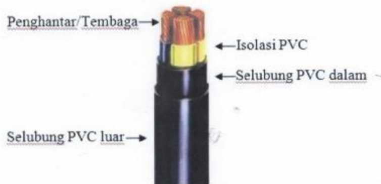
Gambar 2.8 Penampang Kabel Distribusi
