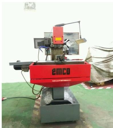
Gambar 3.5. Mesin frais (Milling)
