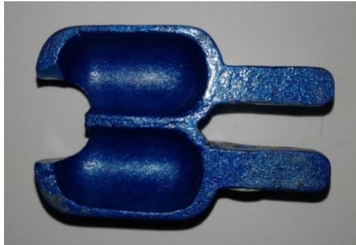
Gambar 3.2 Bucket Turbin Pelton
