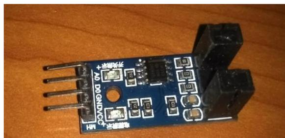
Gambar 3.5 Photo Sensor Interruptor
