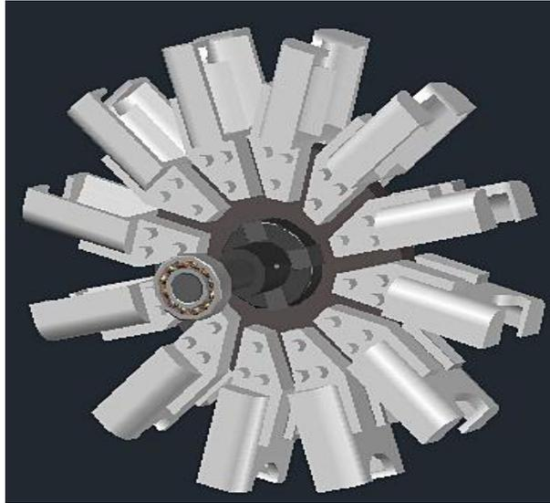
Gambar 3.18 Desain Runner Realistic Autocad 2018
