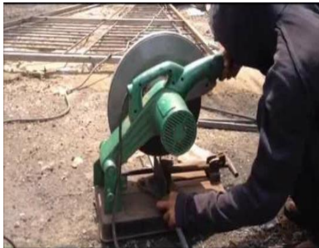
Gambar 4.2 Proses Pemotongan Pipa Steam
