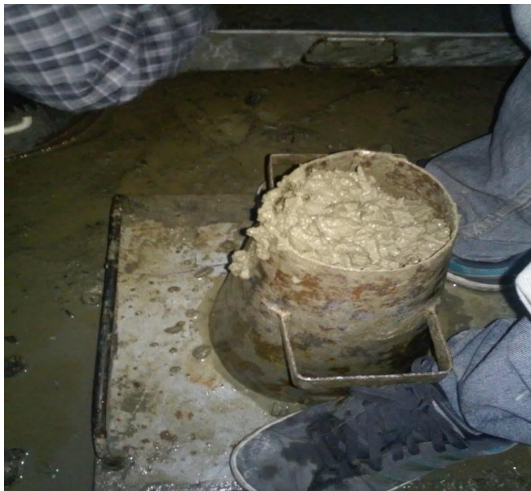
Gambar L6: Proses pengambilan data slump test
