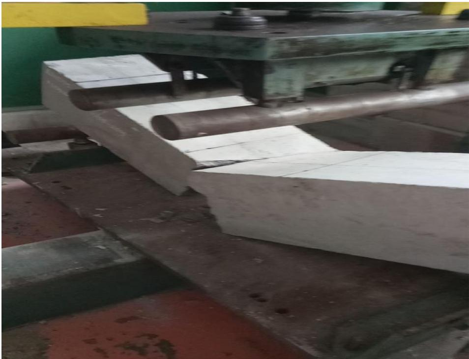
Gambar L24: Pengujian *flexural* beton normal.
