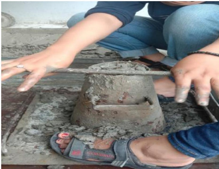
Gambar L12: Pengujian *slump test*.
