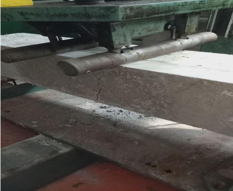
Gambar L25: Pengujian *flexural* beton serat.
