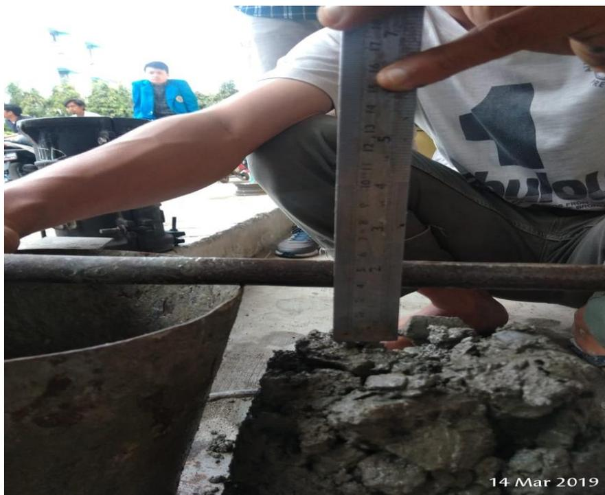
Gambar L15: Pengujian *slump test*.
