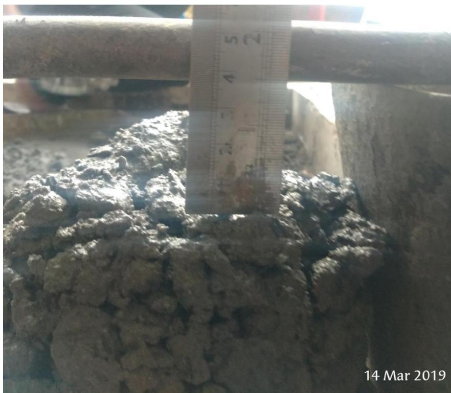
Gambar L24: *Slump test* beton marmer 10% 14 hari sebesar 4 cm.
