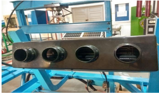
Gambar 2.5. Evaporator AC Mobil (Sumber :Lab UMSU 2019.)
