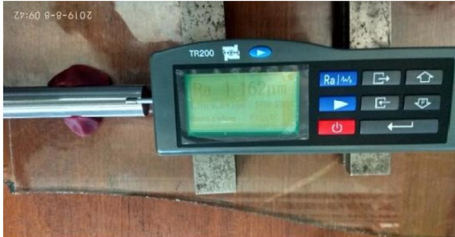
Gambar 4.9 Alat Uji *Roughness Tester*
