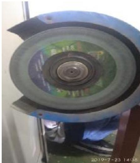
Gambar 3.3 Batu Gerinda ( *Silicon carbide Wheel GC-240 LV*)
