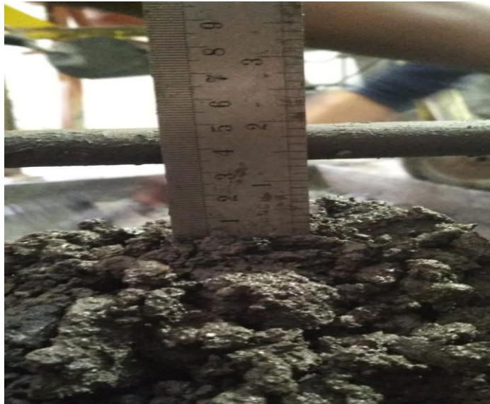
Gambar L9: Pengujian Slump Test .
