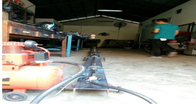
Gambar 3.6 Alat Uji Split Hopkinson Pressure Bar (SHPB)
