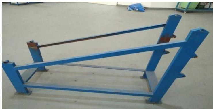
Gambar 4.1. Rangka Mesin *Screw Conveyor*
