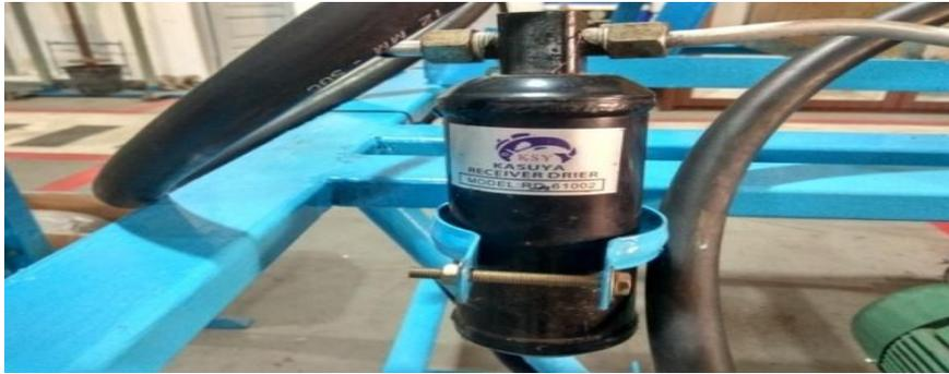
Gambar 3.5 *Receiver Dryer*
