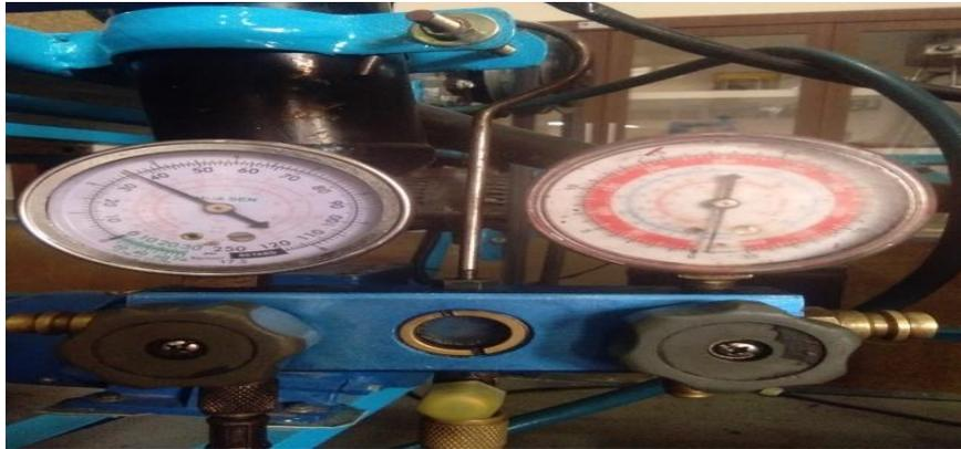
Gambar 3.10 *Manifold Gauge*
