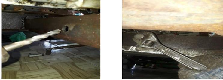
Gambar 56. *I beam axle*
