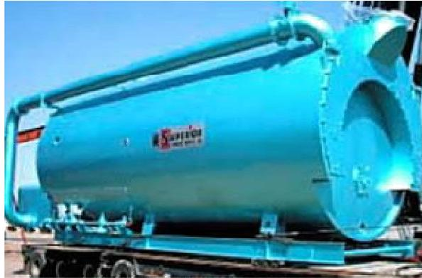
Gambar 2.4 Ketel mobil (*mobile boiler*)
