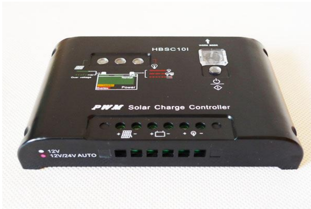
Gambar 2. 6 Solar charge controller (Sumber : Rusman)
