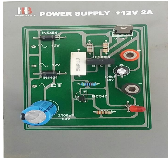
Gambar 3.6 Power Supply ( +12 V / 2A )
