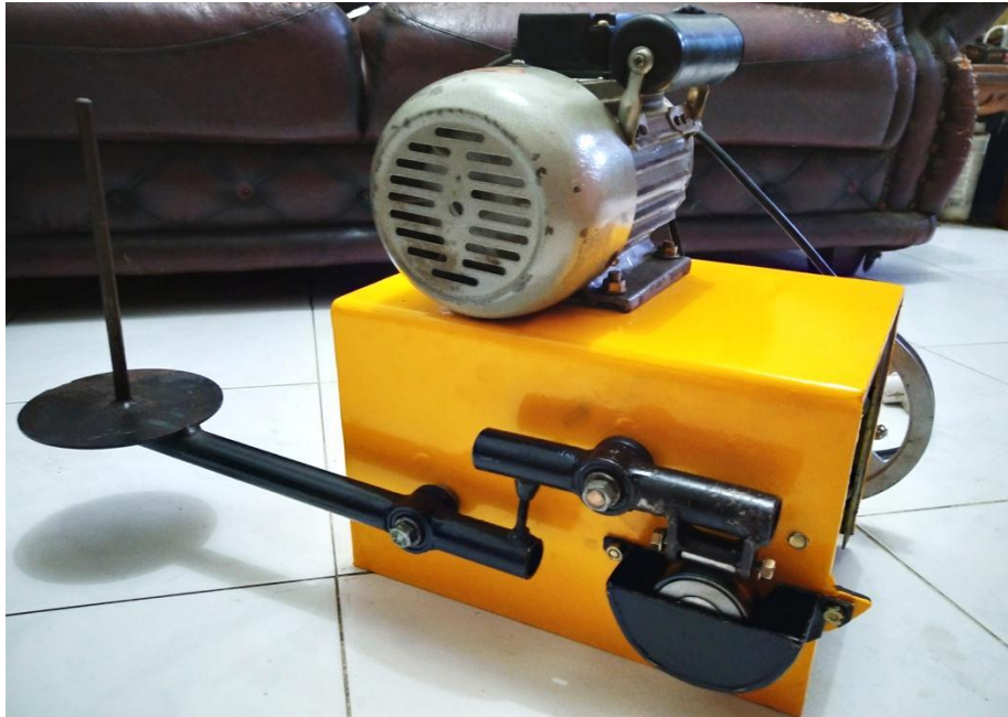
Gambar 4.24. Oil Friction Tester Kapasitas Pembebanan 10 Kgf
