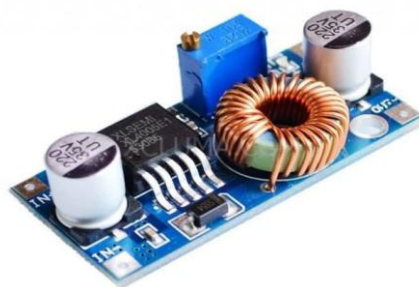
Gambar 3.18. Adaptor DC-DC 5 V (Handika Suparno, 2020)
