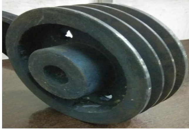
Gambar 3.10 Pully diameter 140 mm
