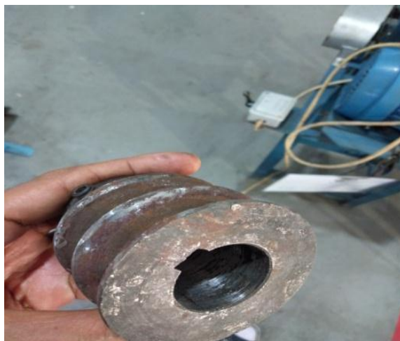
Gambar 3.9 Pully diameter 63 mm
