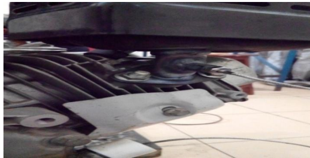
Gambar 3.5 Thermocopel Exhaust manifold
