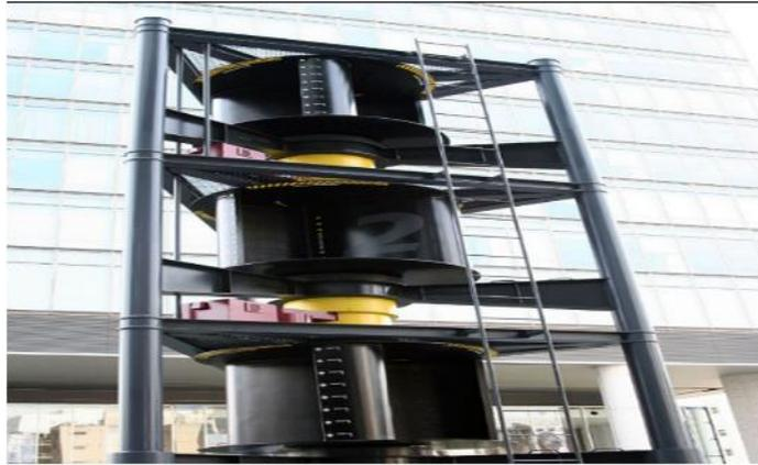
Gambar 2.3 Turbin Angin Savonius(Toshihiro Oimatsu 2006)
